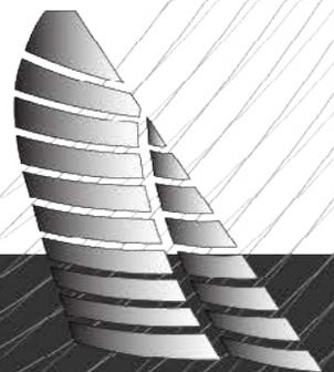
So why not just choose a radial sail every time? There are two major factors that go into the cost of a sail: the fabric and the labor required to build the sail. In both cases a radial sail is more expensive. The laminated fabric is more expensive to produce, and radial sails require more work to manufacture and there is more waste. It is worth remembering that an investment in fabric up front will pay dividends in the long run. It just depends upon your budget.
