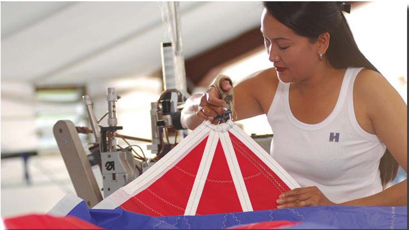
Handwork detailing on a spinnaker clew
