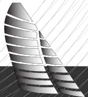
individually created cambered shapes each with its own chord-depth ratio, twist, and maximum depth location. Stacking them on top of each other creates the overall sail shape.
