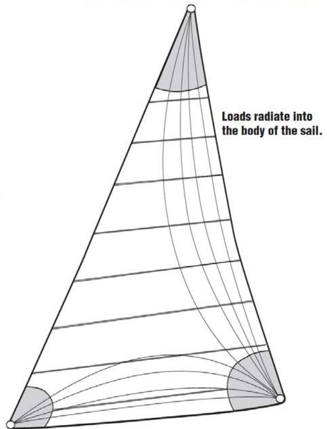
sailing on the wind, a high-aspect sail like a blade jib will have the bulk of the load travel almost directly up the leech of the sail with less stress along the foot. A low-aspect sail like a No. 1 genoa, on the other hand, will have the loads travel more toward the center of
