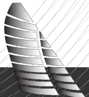
the sail rather than concentrated along the leech. It will also experience greater loads along its foot than the high-aspect sail. By knowing where the loads fall and combining this information with the strength and stretch resistance of the individual yarns, the sail designer can begin to develop an overall picture of an optimal panel configuration.
