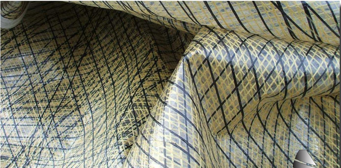
The mylar film is clearly visible in this Carbon Twaron sail
