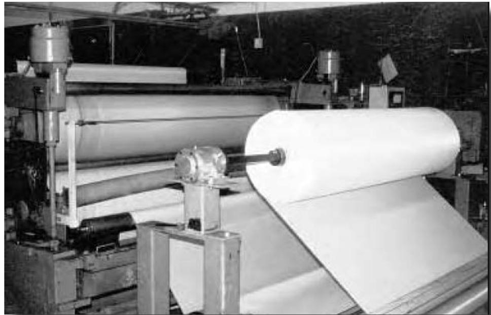
Dacron fabric is passed through a trough of melamine resin to fill the gaps between the yarns and prevent bias stretch.
