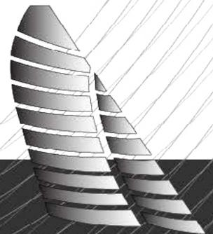
the cloth so that the stronger fibers will bear the bulk of the loads generated by the wind. Both of these fabrics are fill-orientated and should be used for sails where the loads run principally up the leech of the sail. To give you some perspective on how these abstract figures relate to the real world, the 7.62-ounce fabric would be good for a mainsail on a 30-foot daysailer, and the 9.62-ounce fabric would be good for a high-aspect blade jib on a 40-foot racer/cruiser.
